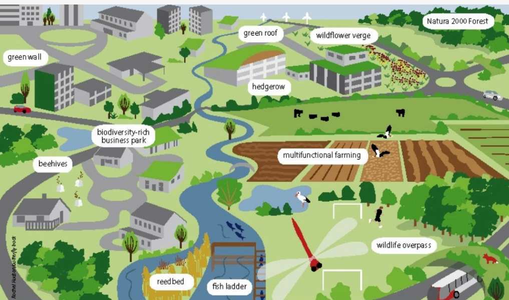
Potential components of a Green Infrastructure
